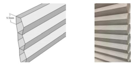
**9.5mm Double Cell** - This fabric has a double cell structure that increases the thermal efficiency of the shade. The headrail on these shades measures 38mm. The minimum reveal depth for inside mount is 38mm (this depth requirement may vary depending on operation type).
